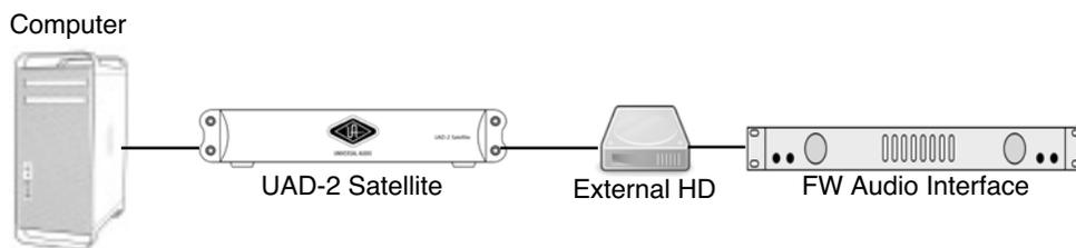
Figure 34. FireWire bus connection via daisy chain
