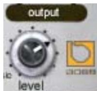
This knob determines the signal level at the output of the plug-in. The range is 0 – 100%.
