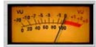
Higher VU levels typically indicate more harmonic saturation, coloration, and/or distortion. However, this will depend on the other control values.
