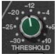
Threshold defines the input level at which expansion or gating occurs. Any signals below this level are processed. Signals above the threshold are unaffected. Threshold is continuously variable from  $-30$  dB to  $+10$  dB.
