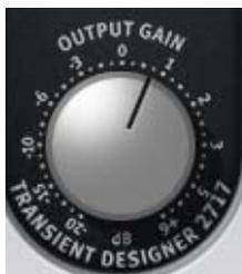
Gain controls the signal level that is output from the plug-in. The available range is from  $-20$  dB to  $+6$  dB. The default value is 0 dB.
