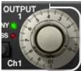
The Output knob controls the signal level that is output from the plug-in.
