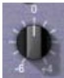
This knob sets the overall gain for the channel. The range for the standard version is continuously variable from  $-6$  dB to  $+4$  dB. The range for the Mastering version is  $\pm 2.5$  dB, in 0.5 dB steps.
