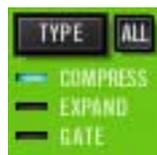
The Type button defines the dynamic nature of the band, allowing each band to function as a compressor, expander, or noise gate, independent of the Type value in the other bands.
