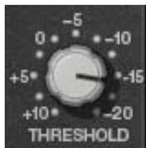
Threshold defines the signal level at which the onset of compression occurs. Incoming signals that exceed this level are compressed. Signals below the level are unaffected.
