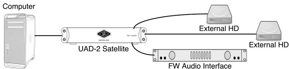
Figure 36. FireWire bus connections using UAD-2 Satellite as a hub
