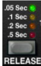
Release sets the amount of time it takes for compression to cease once the input signal drops below the threshold level. Slower release times can smooth the transition that occurs when the signal dips below the threshold, especially useful for material with frequent peaks. However, if you set too large of a Release time, compression for sections of audio with loud signals may extend to lengthy sections of audio with lower signals.
