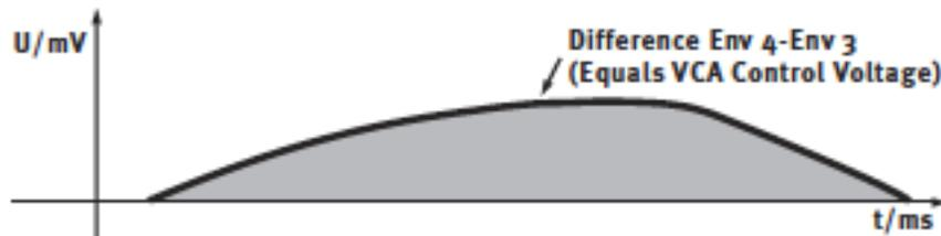
Figure 169. SPL Transient Designer Sustain Control Voltage
