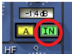
This button enables or disables the Cambridge EQ altogether. You can use this switch to compare the processed settings to that of the original signal, or to bypass the plug-in to reduce UAD DSP load (load is not reduced if “UAD-2 DSP LoadLock” on page 73 is enabled).
