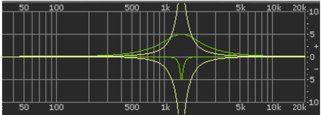
Figure 50. Parametric Type II response
