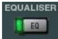
This button activates the equalizer module. The module is active when the button is gray and the green indicator illuminates.
