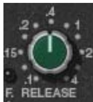
Release sets the amount of time it takes for gate/expander processing to engage once the input signal drops below the Threshold value. The available range is  $0.1$  ms to  $4$  seconds.
