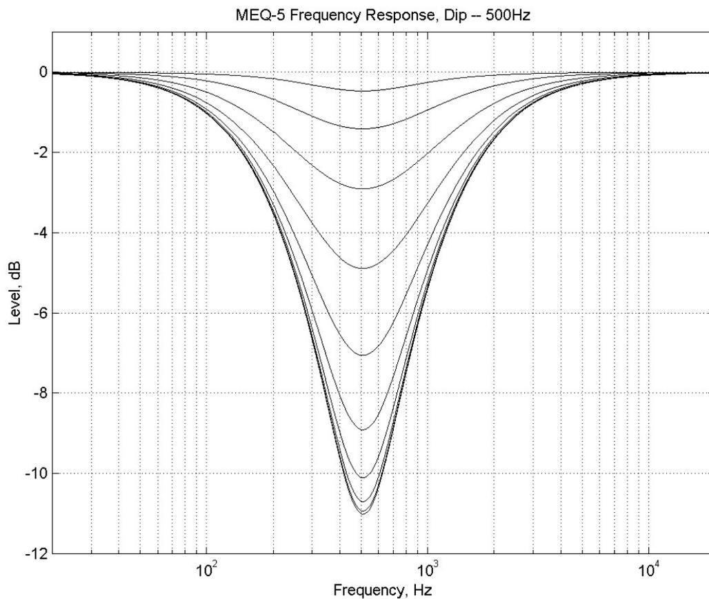
Figure 149. Pultec MEQ-5 Dip Response
