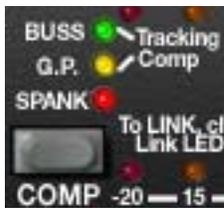
The COMP button defines which compressor mode is active. See "[Compression Processor](#)" on [page 196](#) for a description of the modes.
