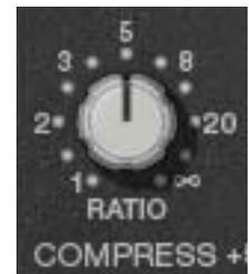
The UAD SSL E Channel Strip compressor offers a continuously variable ratio between 1:1 (no compression) and infinity:1 (limiting).
