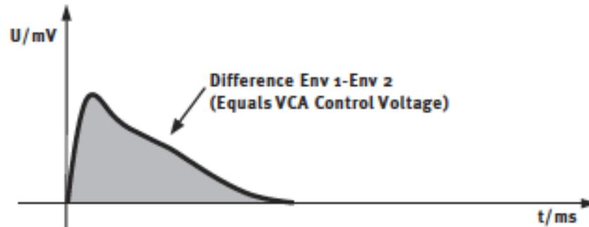
Figure 166. SPL Transient Designer Attack Control Voltage
