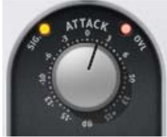
Attack enables amplification or attenuation of the attack of a signal by up to  $\pm 15$  dB.
