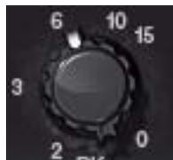
This control determines the amount of gain or attenuation to be applied to the mid band. Up to 15 dB of boost or cut is available.
