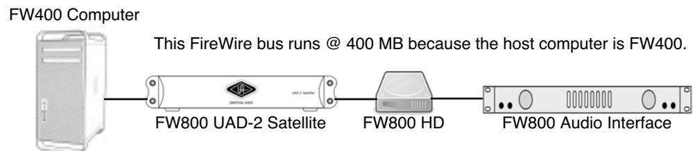
Figure 37. FireWire 400 bus – all devices run at 400 megabits
