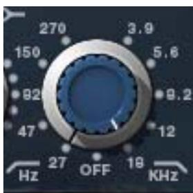
The independent low and high cut filters are controlled by the dual-concentric knobs to the right of the low band (see [Figure 110 on page 315](#)). The controls specify the fixed frequency of the cut filter. The cut filters have an 18 dB per octave slope.
