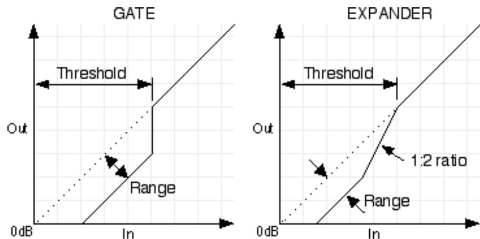
Figure 119. The Neve 88RS Gate/Expander diagram
