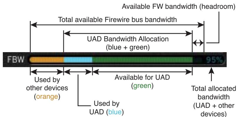
Figure 41. Elements of the UAD FireWire Gauge
