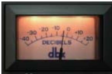
When set to Input, the VU Meter indicates the plug-in input level in dB. When set to Output, the VU Meter indicates the plug-in output level in dB. When set to Gain Change, the VU Meter indicates the amount of Gain Reduction in dB.
