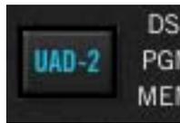
When the button glows blue, UAD plug-ins are active. Click the button to disable the active plug-ins; the button changes to black with blue lettering. New UAD plug-ins can then be added. Click the button again to re-activate all UAD plug-ins.
