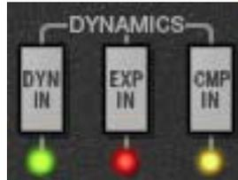
These three buttons determine the status of the dynamics processors.
