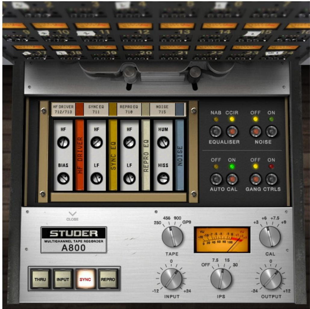
Figure 174. The Studer A800 plug-in window with exposed secondary controls
