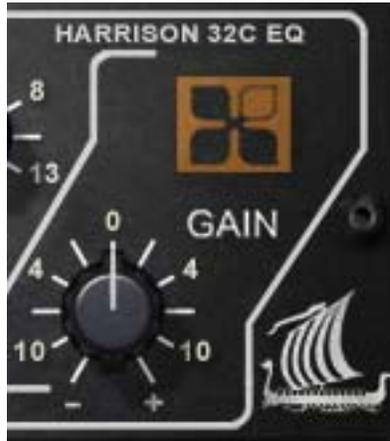
The Gain knob controls the signal level that is output from the plug-in. The default value is 0 dB. The available range is  $\pm 10$  dB.
