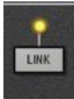
When UAD SSL E Channel Strip is used in a stereo-in/stereo-out configuration, two separate dynamics processors are active (one for each stereo channel). When Link is engaged, the two compressors are constrained so that they both compress by the same amount at any instant.
