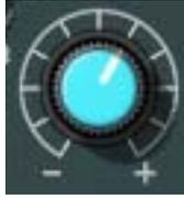
This control determines the amount by which the frequency setting for the HF band is boosted or attenuated. The available range is  $\pm 20$  dB.
