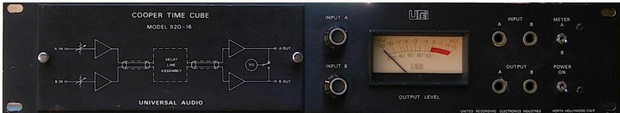
Figure 58. The original Cooper Time Cube hardware front panel
