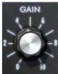
The non-linear modeling of Drive characteristics is extremely DSP-intensive. For this reason, Drive is not available on the SE version of UAD Moog Filter. In UAD Moog Filter SE, the parameter is named Gain instead of Drive, and is a straight (non-modeled) input gain control.
