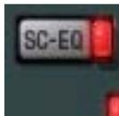
This control enables the UAD Neve 88RS sidechain function. When sidechain is active, signal output from the EQ module is removed from the audio path and is instead routed to control the dynamics module.
