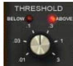
The available range is from  $-55$  dB to 0 dB. The numbers on the graphical interface indicate volts, as on the original hardware.
