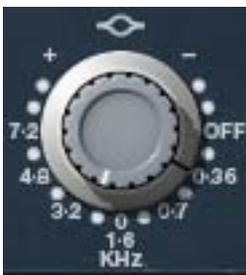
The midrange band is controlled by dual-concentric knobs, delivering smooth semi-parametric midrange equalization.
