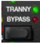
This black button is a multifunction control. Clicking the button repeatedly cycles through Tranny, Bypass, and Tranny Off modes. The currently active mode is indicated by the adjacent LED's.
