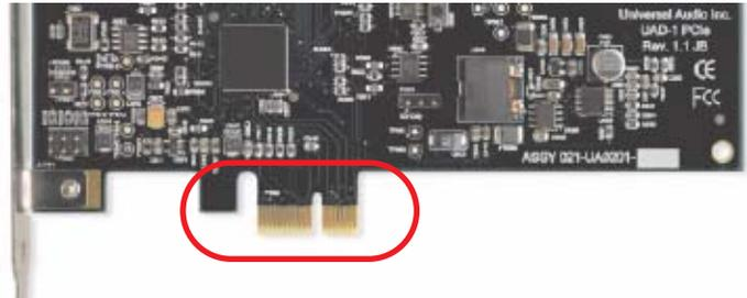
Figure 1. PCI and PCIe connectors are incompatible
