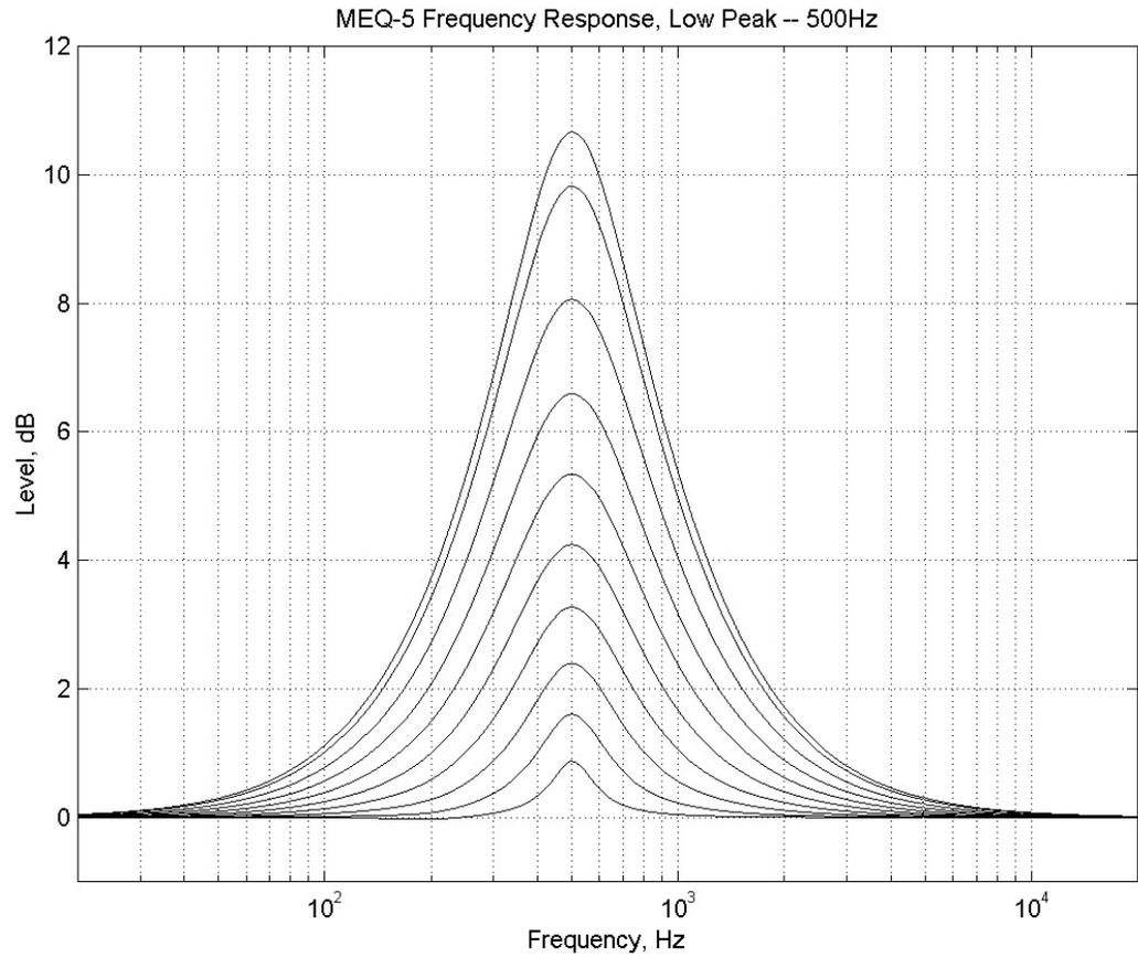
Figure 148. Pultec MEQ-5 Low Peak Response
