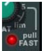
The Fast mode switch defines the attack time (the duration between the input signal reaching the threshold and processing being applied) of the limiter and compressor.
