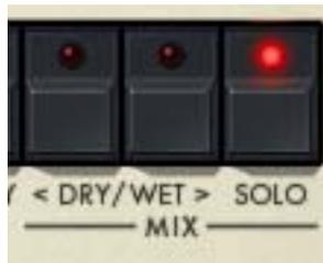
The Dry, Wet, and Solo parameters control the effect mix in the plug-in. These controls are not available in the original hardware.
