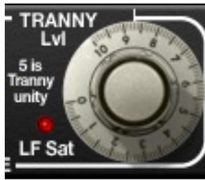
This control determines the amount of Tranny processing (see “The Tranny Processor” on page 195 for a detailed description). Higher values make the Tranny effect more prominent. Increasing the Tranny level also increases the signal THD (see “THD Indicators” on page 198), and the sensitivity of the Warmth processor (page 199). A value of 5 is the unity setting.
