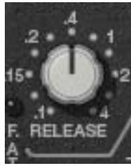
Release sets the amount of time it takes for gain reduction to cease once the input signal drops below the threshold level. Longer release times can smooth the transition that occurs when the signal dips below the threshold, which is especially useful for material with frequent peaks. However, if you set the Release time too long, the gain reduction imposed by loud sections of audio may initially reduce the level of subsequent sections of audio with lower signals.
