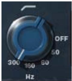
This knob specifies the fixed frequency of the Low Cut filter. This filter has an 18 dB per octave slope.
