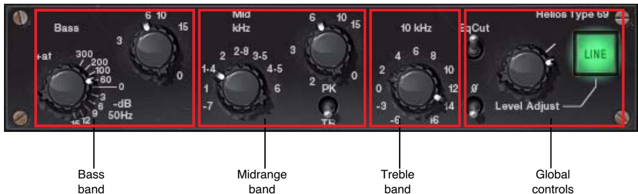
Figure 86. Helios 69 band control layout
