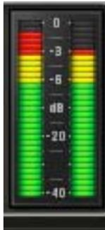
The stereo peak Output Meter displays the signal level at the output of the plug-in. The displayed range is from  $-40$  dB to  $0$  dB.
