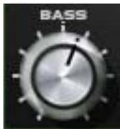
This knob controls the low frequency response in the tape echo portion of the signal. It does not affect the dry signal or the reverb signal. This is a cut/boost control; it has no effect when in the 12 o'clock (straight up) position.
