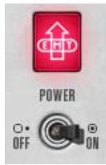
This toggle switch enables or disables EMT 140. You can use it to compare the processed settings to the original signal, or to bypass the plug-in which reduces (but not eliminates) the UAD DSP load (unless “UAD-2 DSP LoadLock” on page 73 is enabled). The red EMT power indicator glows brighter when the plug-in is enabled.
