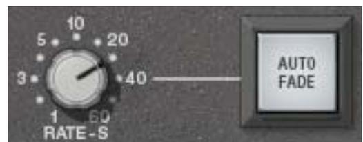
The Fade function processes the signal at the output of the compressor. The fade signal level that is output has an exponential curve.
