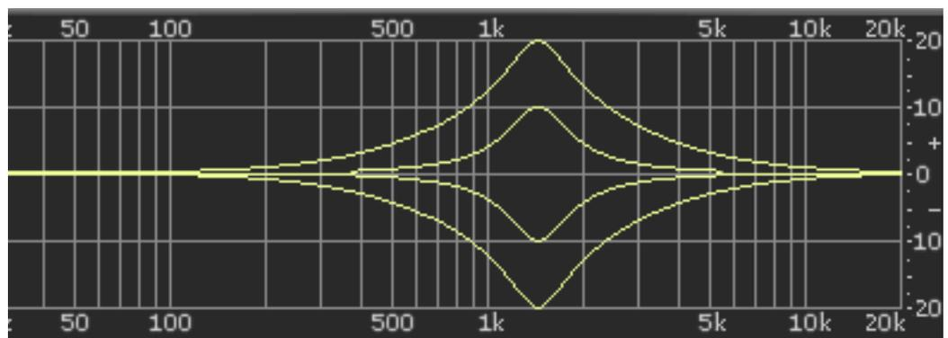
Figure 49. Parametric Type I response
