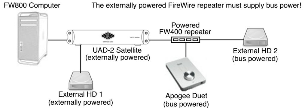
Figure 43. Proper connection of bus powered FireWire devices
