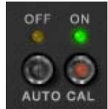
When Auto Cal (Automatic Calibration) is ON in the plug-in, these calibration controls (see [Figure 175 on page 514](#)) are automatically adjusted to the calibrated values whenever the Tape Type, Tape Speed, and Emphasis EQ are modified. After Auto Calibration occurs, the automatically adjusted parameters can then be modified to any value if desired.
