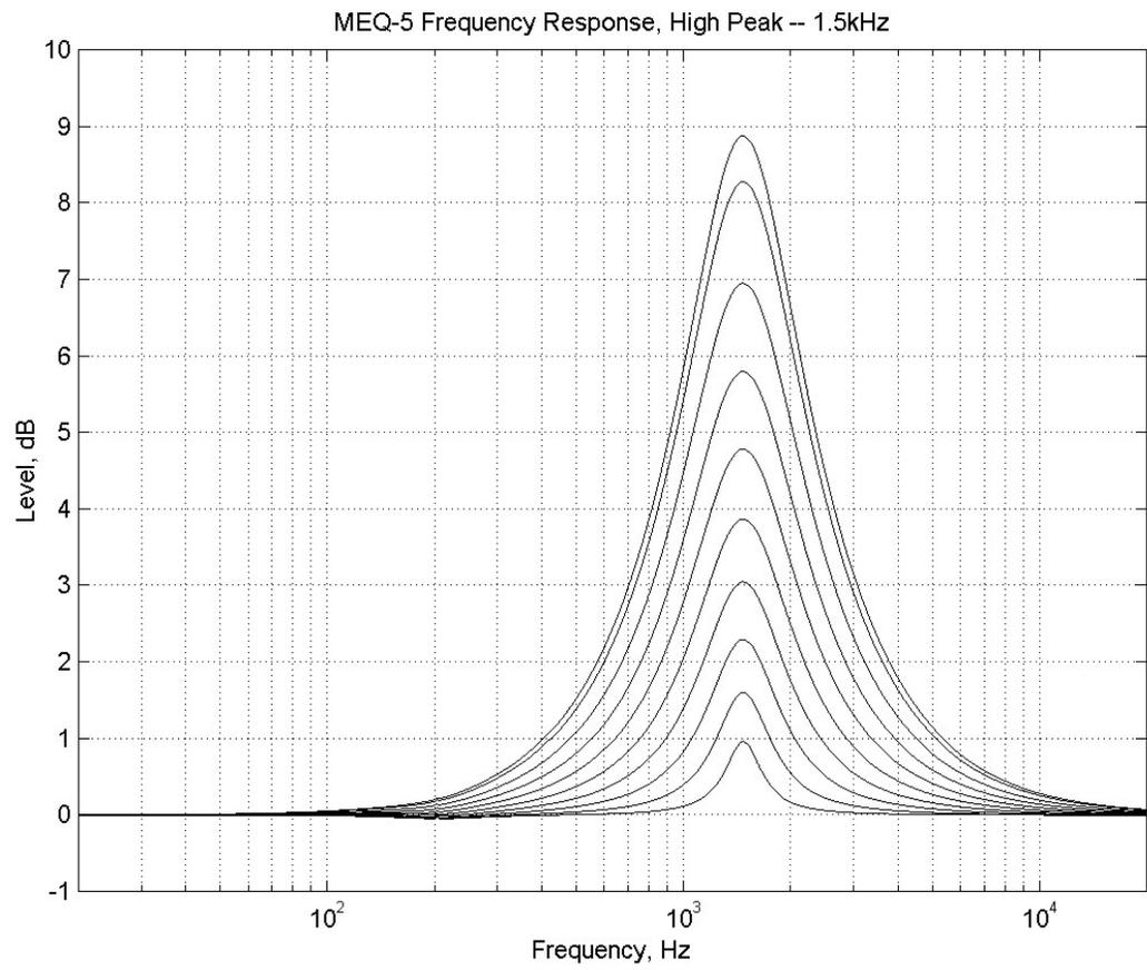
Figure 150. Pultec MEQ-5 High Peak Response
