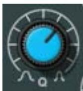
The Q (bandwidth) control defines the proportion of frequencies surrounding the HMF band center frequency to be affected by the band gain control. The filter slopes get steeper (narrower) as the control is rotated clockwise. The available range is 0.4 to 10.
