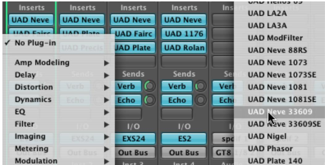
Figure 17. Launching a UAD Powered Plug-In in Apple Logic Pro
