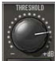
This parameter determines the threshold level for the onset of compression. Incoming signals that exceed this level are compressed. Signals below the level are unaffected.
