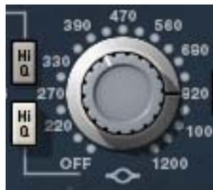
The low-midrange band delivers smooth low-mid frequency peak equalization with a choice of two bandwidths. The inner knob controls the band gain, and the outer ring selects the frequency or band disable.
