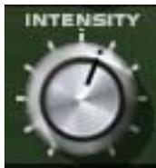
This knob controls the repeat level (feedback) of the echo signal. Rotating the control clockwise increases the number of echoes. Higher values will cause self-oscillation; the exact position is program and Mode dependent.
