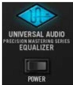
The Power Switch determines whether the plug-in is active. This is useful for comparing the processed settings to the original signal, or to bypass the plug-in to reduce the UAD DSP load (load is not reduced if “UAD-2 DSP LoadLock” on page 73 is enabled).
