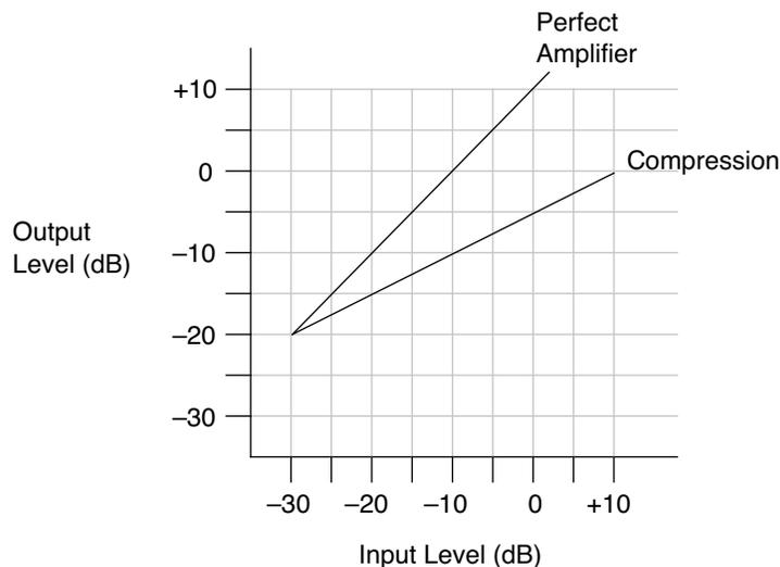
Figure 87. Input and output characteristics of a compressor and perfect amplifier
