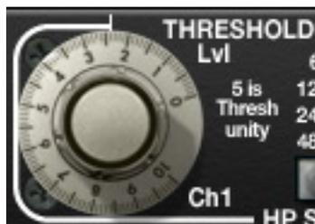
This knob enables manual threshold control of the FATSO compressor. Higher values lower the threshold, and therefore increase the amount of compression. A value of 5 is the unity setting.
