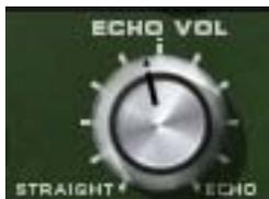
This control determines the volume of the echo effect. Rotate the control clockwise for louder echo. Reducing the control to its minimum value will disable the echo.
