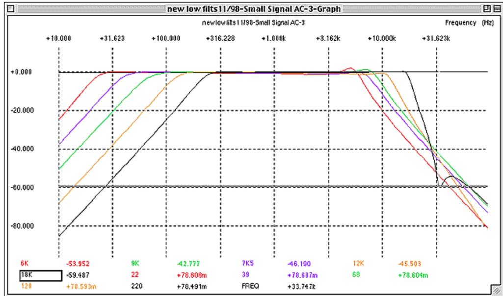
Figure 104. High Pass and Low Pass filter response curves (standard version)
