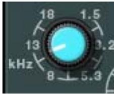
This parameter determines the HF band center frequency to be boosted or attenuated by the band Gain setting. The available range is 1.5 kHz to 18 kHz.
