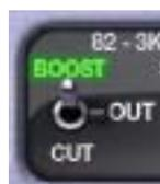
This three-position toggle switch determines whether the frequency band will be boosted, cut, or disabled altogether. The amount of boost or cut to be applied to the band is determined by the [Band Gain](#) control.
