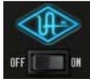
The Power switch determines whether the plug-in is active. This is useful for comparing the processed settings to the original signal or bypassing the plug-in to reduce the UAD DSP load (load is not reduced if “UAD-2 DSP LoadLock” on page 73 is enabled).
