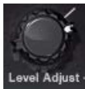
This control adjusts the signal output level of Helios Type 69. This may be necessary if the signal is dramatically boosted or reduced by the EQ settings. The available range is -20 dB to +10 dB.
