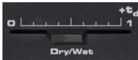
The Dry/Wet slider control determines the balance between the original and the processed signal. The range is from 0% (dry, unprocessed) to 100% (wet, processed signal only).
