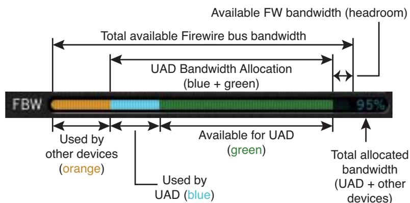
Figure 14. Elements of the UAD FireWire Gauge
