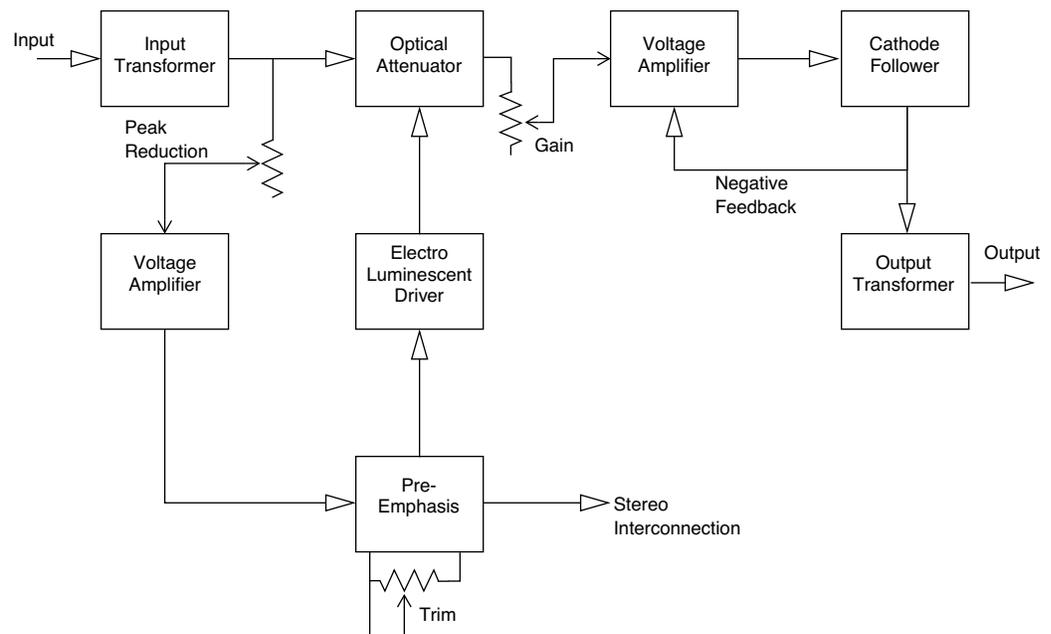
Figure 89. LA-2A signal flow
