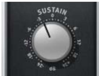
Sustain enables amplification or attenuation of the sustain of a signal by up to  $\pm 24$  dB.
