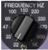
This control defines the center frequency (Bell mode) or edge frequency (Shelf mode) for the band. Each band provides a wide range of specially tuned overlapping and interleaving frequency choices. The available frequencies for each band are listed in [Table 18](#) below.
