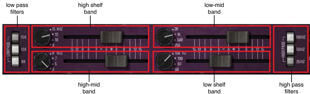
Figure 177. Trident A-Range band control layout
