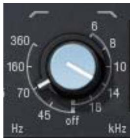
The independent low and high cut filters are controlled by the dual-concentric knobs to the right of the low band. The controls specify the fixed frequency of each cut filter.
