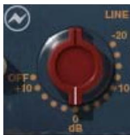
The Input Gain control sets the level at the input of the plug-in. The range is from  $-20$  dB to  $+10$  dB.
