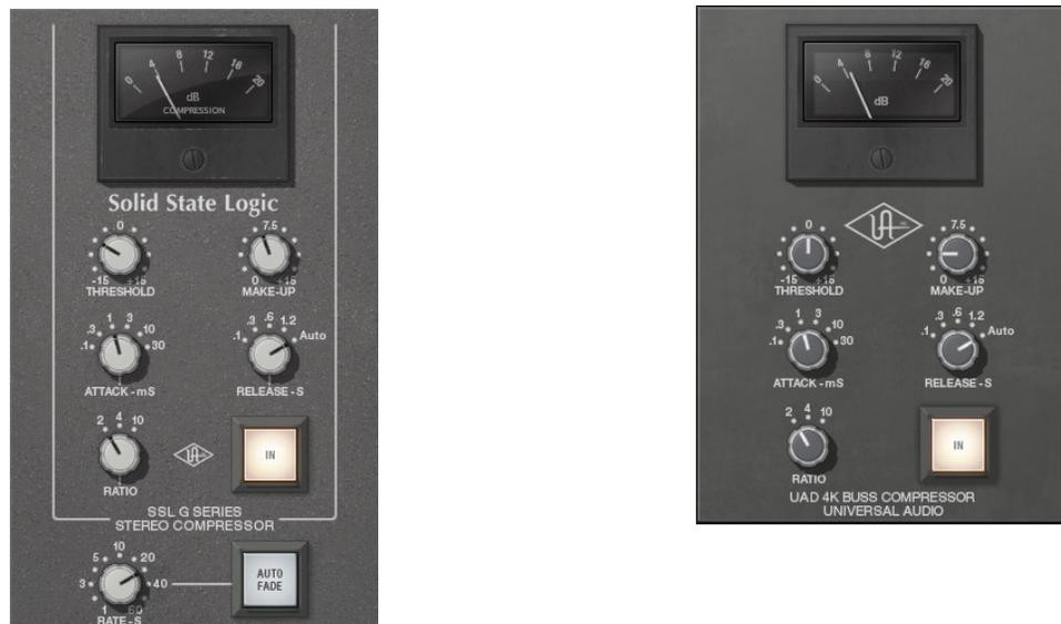
Figure 172. The SSL G and 4K Bus Compressor plug-in windows
