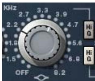
The high-midrange band delivers smooth high-mid frequency peak equalization with a choice of two bandwidths. The inner knob controls the band gain, and the outer ring selects the frequency or band disable.
