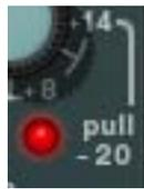
The -20 dB switch increases the sensitivity of the limiter/compressor by lowering the range of the available threshold values. When -20 dB mode is active, the threshold range is 0 dB to -30 dB. When -20 is inactive, the threshold range is +20 dB to -10 dB.
