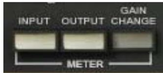
The Meter buttons define the mode of the VU Meter. The buttons do not change the sound of the signal processor. The active button has a darker appearance when compared to the inactive buttons.
