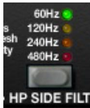
Filter regulates the cutoff frequency of the filter on the compressor's control signal sidechain. When active, frequencies below the filter value are not passed to the sidechain. Values of 60 Hz, 120 Hz, 240 Hz, 480 Hz, and Off are available. The filter slope is 6 dB per octave. When the compressor is disabled, Filter has no effect and its LED turns off. When the compressor is enabled, Filter returns to its original value.
