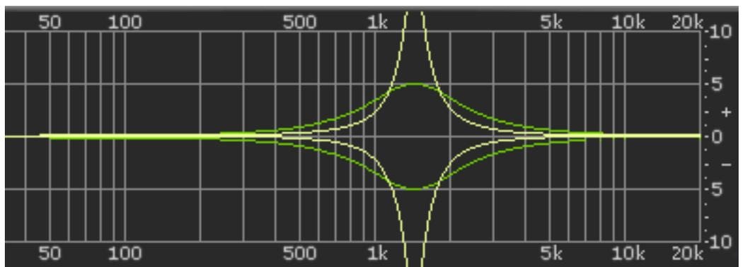
Figure 51. Parametric Type III response
