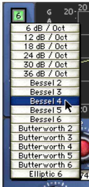
The Cut Type menu determines the sound of the low and high cut filters. To view the Cut Type menu, click and hold the green cut type button.
