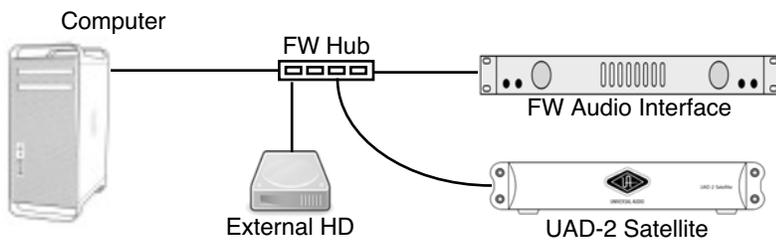
Figure 33. FireWire bus connections via a hub
