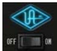
The Power switch determines whether the plug-in is active. This is useful for comparing the processed settings to the original signal or bypassing the plug-in to reduce the UAD DSP load (load is not reduced if “UAD-2 DSP LoadLock” on page 73 is enabled).
