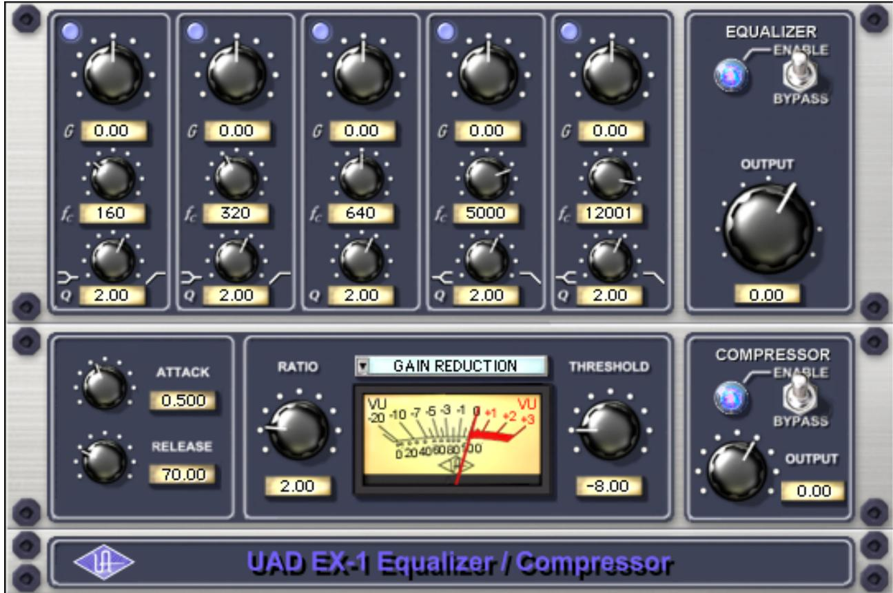
Figure 61. The EX-1 EQ/Compressor plug-in window
