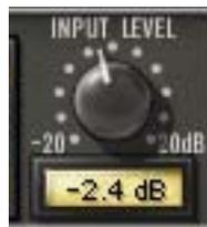
Input controls the signal level that is input to the plug-in. Increasing the input may result in more compression, depending on the values of the Threshold and Ratio parameters.
