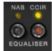
NAB or CCIR curves can be selected when the Tape Speed is 7.5 or 15 IPS. When the Tape Speed is 30 IPS, neither value is available (the LEDs are dimmed) because the EQ is fixed with the AES emphasis curve.
