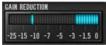
The Gain Reduction meter provides a visual indication of how much attenuation (compression) is occurring. Signal peaks are held for 3 seconds before resetting.
