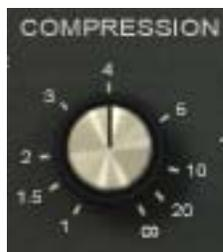
The Compression parameter determines the ratio for the compressor. Less compression occurs at lower values. The available range is continuous, from 1.00:1 to Infinity:1.
