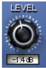
This control adjusts the signal output level of Cambridge EQ. This may be necessary if the signal is dramatically boosted or reduced by the EQ settings. The available range is  $\pm 20$  dB.
