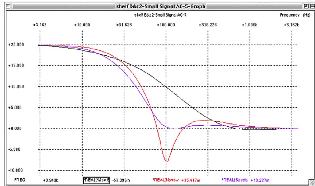
Figure 103. Effect of Bandwidth control on response curve in Shelf mode
