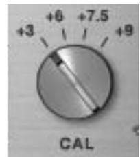
The record, repro, and sync gain trims found on the A800 channel cards are not present on the plug-in. Instead (when "Auto Cal" on page 512 is enabled), these controls are amalgamated into this single Cal Level gain control.
