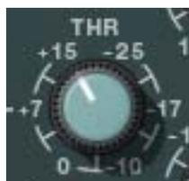
Threshold defines the input level at which expansion or gating occurs. Any signals below this level are processed. Signals above the threshold are unaffected.
