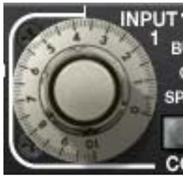
The Input knob defines the signal level going into the plug-in. Higher levels result in a more saturated signal. Levels above 0 VU provide dramatically higher distortion characteristics, especially when clipped (as indicated by the Pinned LED). See [THD Indicators](#) below.
