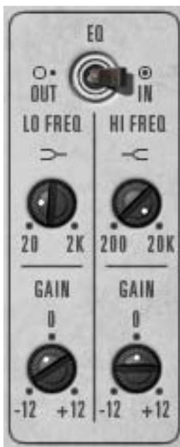
This group of parameters contains the controls for EMT 140's onboard utility equalizer. It is a two band (low and high) shelving EQ that uses analog-sounding algorithms for great tonal shaping options.
