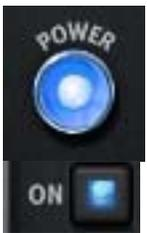
The On and Power switches determine whether the plug-in is active. Click the On or Power switches to change the state. On and Power illuminate when the plug-in is active.
