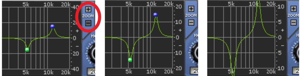
Figure 46. Vertical resolution of the Response Curve can be changed with the Zoom buttons
