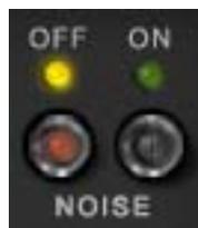
The Noise Enable buttons are a global enable/disable control for the individual hum and hiss components of the A800 model. The amount of hum and hiss noises are continuously variable and are set with the [Hum Noise](#) and [Hiss Noise](#) controls ([page 515](#)). Click the Noise buttons to alternate between OFF and ON.
