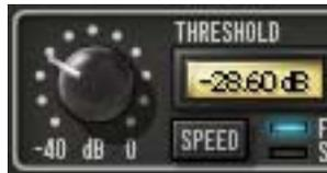
Threshold controls the amount of de-essing by defining the signal level at which the processor is activated. Rotate Threshold counter-clockwise for more de-essing.
