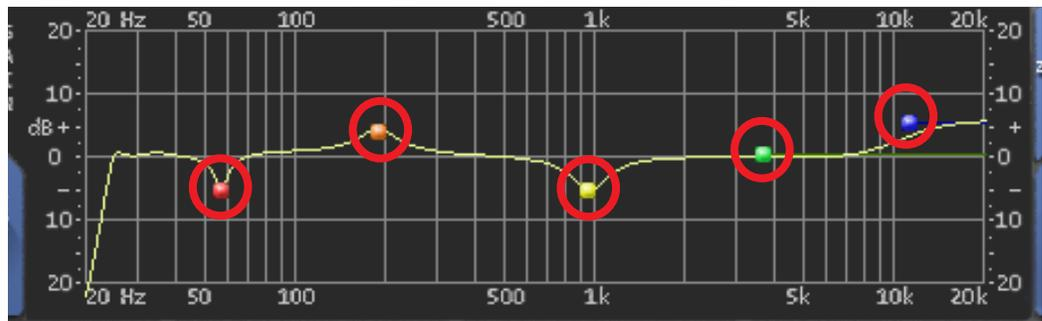
Figure 47. The Curve Control Bats can be used to control EQ band frequency, gain, and Q
