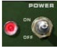
This switch determines whether the plug-in is active. This is useful for comparing the processed settings to the original signal, or to bypass the plug-in to reduce the UAD DSP load. Toggle the switch to change the Power state.
