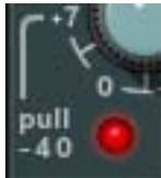
The  $-40$  dB button increases the sensitivity of the gate and expander by lowering the range of the available threshold values. When  $-40$  dB mode is active, the threshold range is  $-25$  dB to  $-65$  dB. When  $-40$  is inactive, the threshold range is  $-25$  dB to  $+15$  dB.
