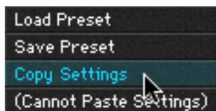
Settings can be copied and pasted directly between UAD plug-ins (within the compatibility guidelines) without using the interim step of creating a preset file.
