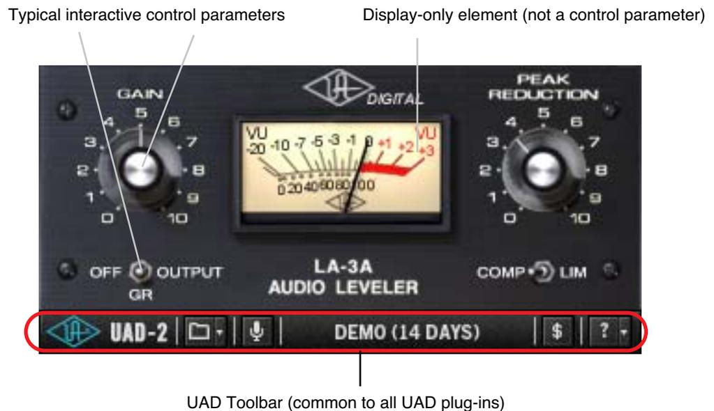
Figure 18. A typical UAD plug-in window
