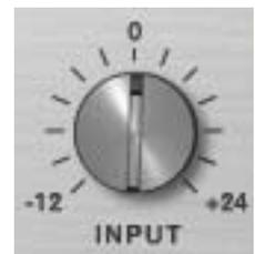
Just like real magnetic tape, lower Input levels will have a cleaner sound, while higher levels result in more harmonic saturation and coloration.
