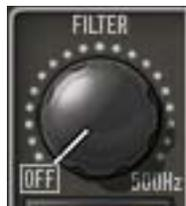
Filter regulates the cutoff frequency of the filter on the compressor's control signal sidechain. Removing low-frequency content from the sidechain can reduce excessive gain reduction and/or “pumping” on bass-heavy audio signals without reducing bass content of the audio signal itself.
