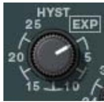
The Hysteresis knob sets the difference in threshold for signals that are either rising or falling in level. Signals that are rising in level are passed when the level reaches the threshold value plus the hysteresis value. Signals that are falling in level are not passed at the lower threshold level. Up to 25 dB of hysteresis is available. See [Figure 120 on page 341](#).
