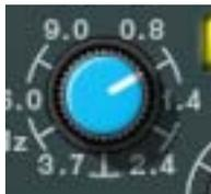
This control determines the HMF band center frequency to be boosted or attenuated by the HMF Gain setting. The available range is 800 Hz to 9 kHz.
