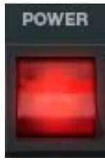
The Power switch determines whether the plug-in is active. This is useful for comparing the processed settings to the original signal or bypassing the plug-in to reduce the UAD DSP load (load is not reduced if “UAD-2 DSP LoadLock” on page 73 is enabled).
