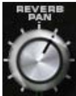
Reverb Pan determines the placement of the reverb signal in the stereo panorama when the plug-in is used in mono-in/stereo-out and stereo-in/stereo-out configurations. When the RE-201 is used in a mono-in/mono-out configuration, this control is disabled.
