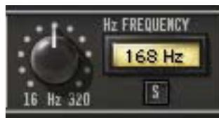
Through filter isolation of the original bass content, the Hz Frequency parameter defines the cutoff frequency for the enhancement process. Frequencies below this value are enhanced by the processor. The available range is 16 Hz to 320 Hz.
