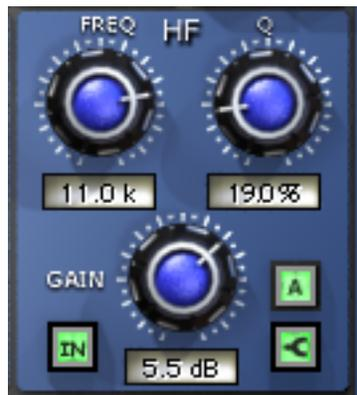
Figure 48. The EQ Band controls
