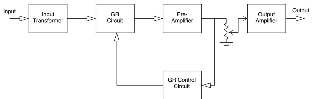
Figure 91. 1176LN signal flow
