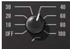
The high-pass filter is useful for reducing low frequency content. It is a global filter; it always affects both left and right channels, regardless of the active mode. See [Table 30](#) below for available settings.
