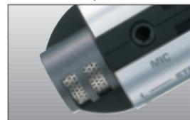
While compact, a stereo microphone is built in that allows you to achieve natural stereo capture through X/Y-type allocation.
