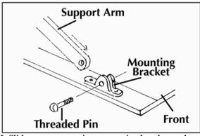
5. Slide support arm into mounting bracket and secure with threaded pin.
