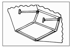
8. Fabric awning should appear as shown above (upside down) to be ready for mounting/installation.
