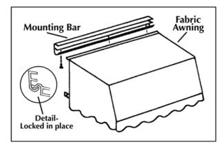
2. Raise front of Awning and insert top trim into mounting bar. Align holes and secure Top Trim with small screws from bottom side.
