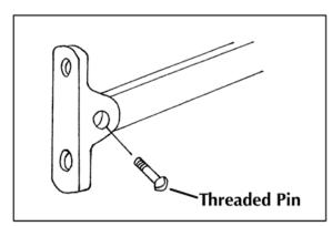
7. Threaded pin will be removed later & re-installed through a grommeted tab.
