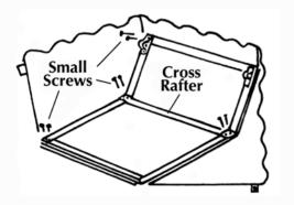
4. Repeat steps 2 & 3 on other awning rafter as shown. Secure cross rafter with small screws.
