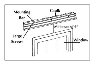
1. Install mounting bar with large screws a minimum of 6" above window. Be sure bar is level and centered over opening. Caulk top of bar against wall. Be sure window opens under Awning before installing all screws.
