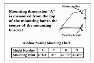
4. Mounting points on this chart should be accurate. However, you may check the proper angle of the support arms by placing a level on them.
