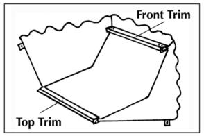
1. Layout fabric awning with top & front trim facing up. Assembly should be done on a clean, dry surface.
