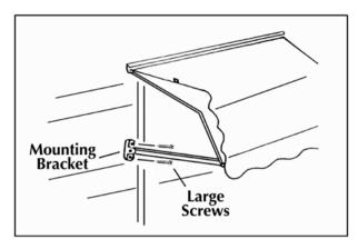
3. To secure the support arms to house, check the mounting chart in step 4 for model number and correct mounting point. Secure mounting brackets to house with large screws.
