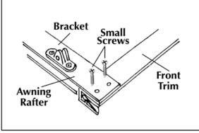
2. Attach awning rafter with pre-attached bracket to front trim using small screws.
