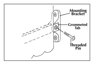
5. After mounting brackets have been secured to the house, remove the threaded pins and re-insert them through grommeted tabs then back into the brackets to secure the Awning sides.
