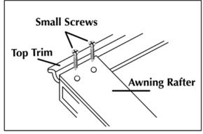
3. Attach the other end of awning rafter to top trim using small screws.
